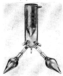
Standard lyophilizing unit with a capacity of 400 ml. is being produced by Wakefield Industries Inc. Because of the many requests for custom-made lyophilizing units, Wakefield decided to produce this design as a standard item. The apparatus is made of Pyrex glass tubing and is furnished with 4 receiving flasks
